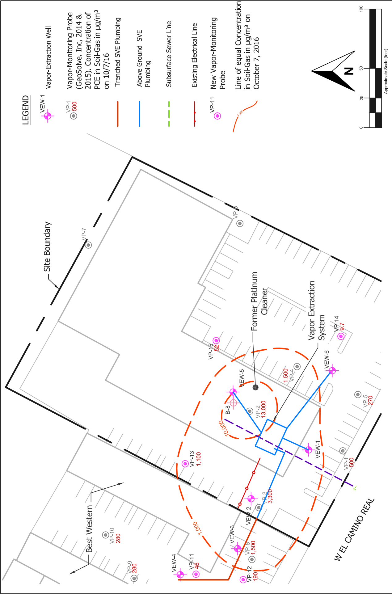
ISO CONCENTRATION MAP FOR PCE IN SOIL-GAS FROM 15 FEET TO 25 FEET
